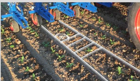
Due to its slanted positions the rotor always cuts at the **right angle** to the crop row.
